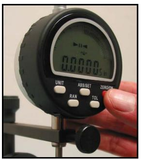
5. Press the RAN (Range) three times to put the indicator into the "TIR/FIM" mode.
