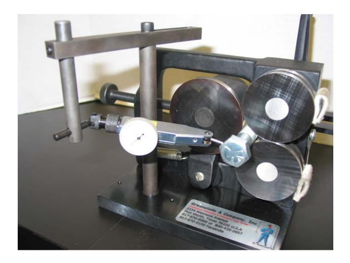
2. Perform the above procedure for loading the fastener. Locate the stylus of the test indicator to the face you are trying to measure and rotate the handle to observe total indicator movement.
